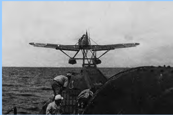
The aircraft carried two incendiary 168 pound bombs and a crew of two.
